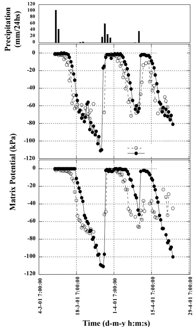
Figure 2. Soil matrix potential response to the pluviometric events (mm/24hs), obtained the tensiometer and by the Watermark (GMS) (kPa), for 15 cm depth, for plots B and D.
