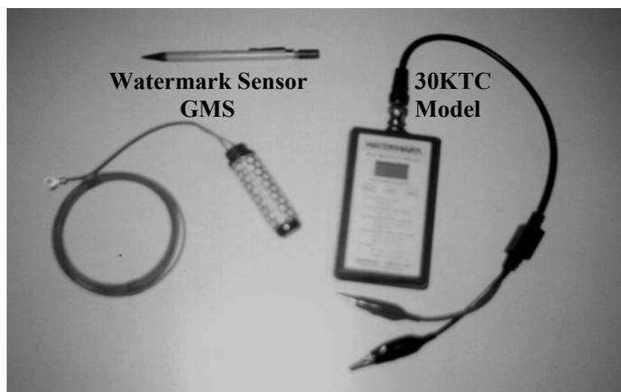
Figure 1. Watermark sensor (GMS) developed by Irrometer Co. On the left is shown the sensor with the cables, while on the right is shown the gauge used in this study (30KTC model).
