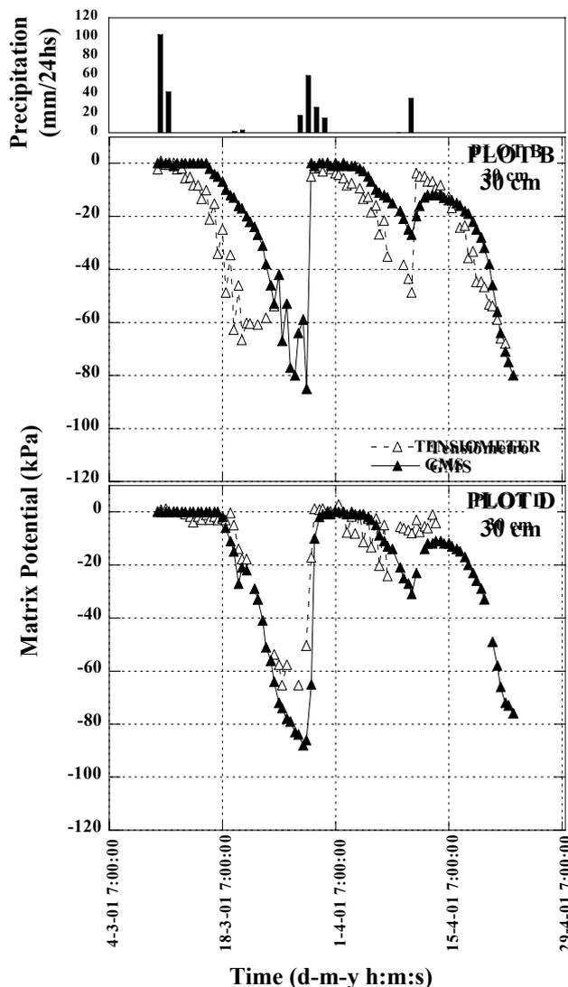
Figure 3. Soil matrix potential response to the pluviometric events (mm/24hs), obtained the tensiometer and by the Watermark (GMS) (kPa), for 30 cm depth, for plots B and D.
