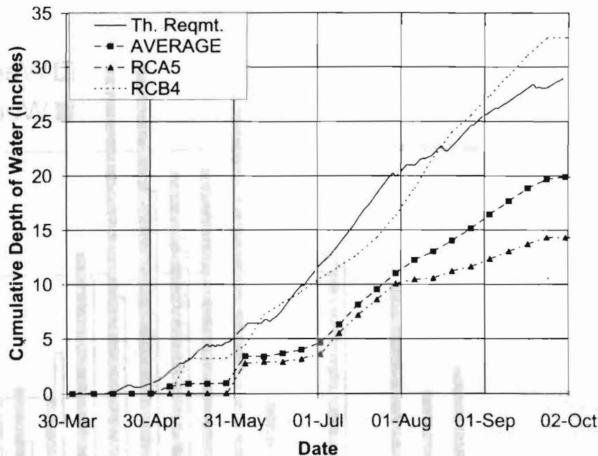
Figure 3. Comparison Among Theoretical Irrigation Requirement and Average, Maximum (RCB4), and Minimum (RCA5) Actual Applications With Respect to Time.
