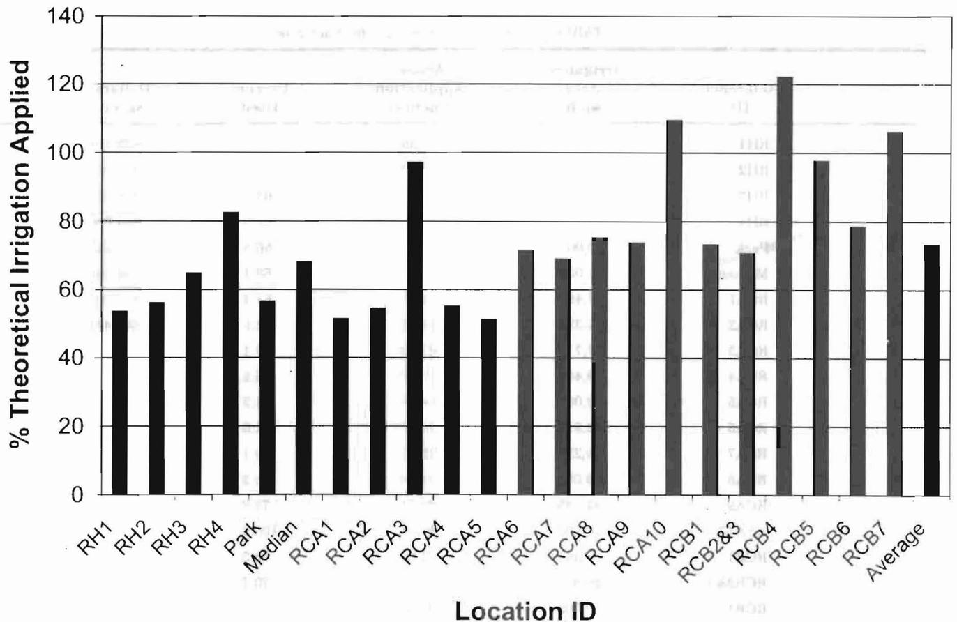
Figure 2. Ratio of Actual Application to Theoretical Requirement Expressed as a Percentage for Each Sprinkler Clock With a Watermark Electronic Module and Granular Matrix Sensors.
