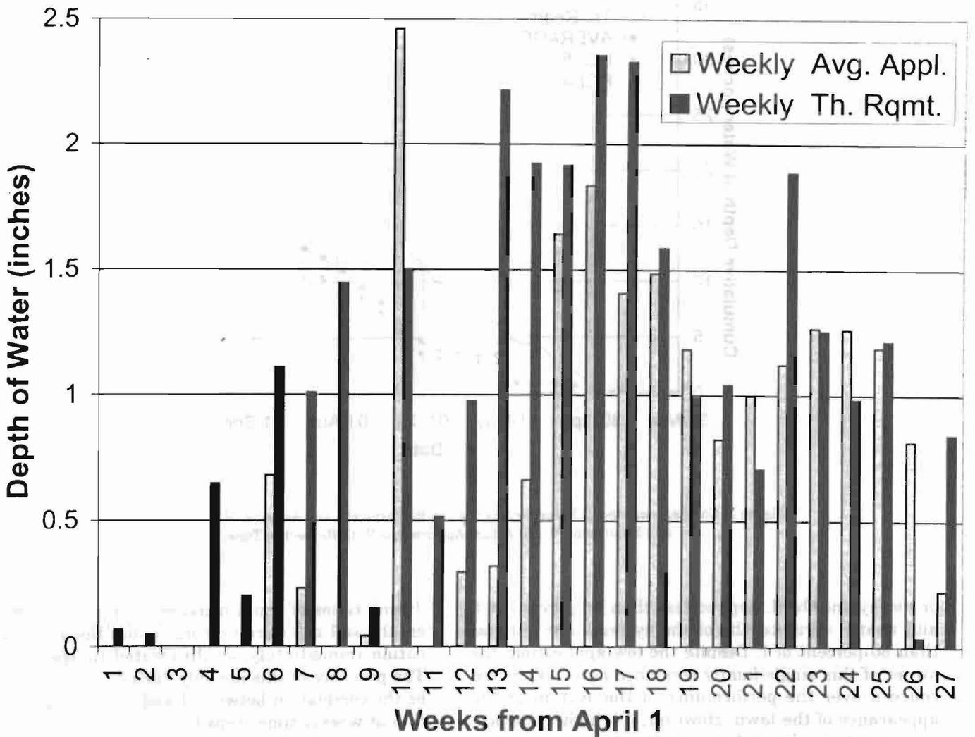
Figure 4. Comparison Between Site-Averaged Applications and Theoretical Irrigation Requirement on a Weekly Time Step.
