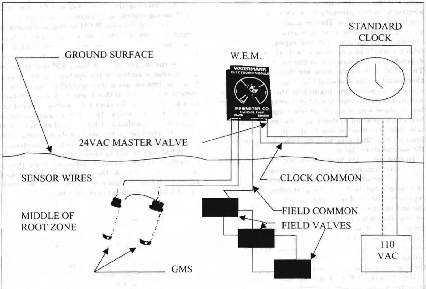
Figure 1. Schematic of Typical Automated Irrigation Installation.
