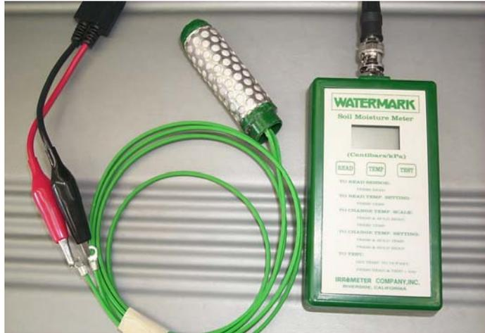
*Electrical resistance block soil moisture probe with hand-held reader*
