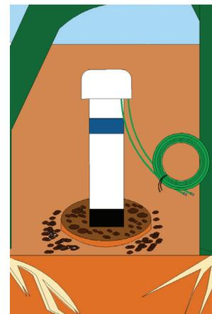
**Step 4:** Repeat steps 1–3 for each of the 12-, 24-, and 36-inch sensors. Space the sensors about 1 foot apart. Place a flag at the sensor location and at both the top and bottom ends of its crop row to make finding the sensor set easier.
