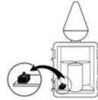
**Base Node** — Cover the solar panels of the Base Node and slide the power switch inside the capacitor housing to 'OFF'.
