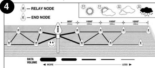
placed at the extremities of the system or located so as to provide in-fill near relaying Nodes. (see Figure 4)
