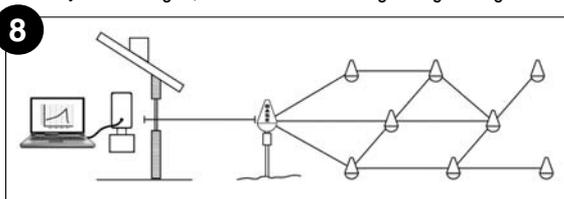
associated to the fully charged Base outside. Take the PC Link to within 2' of the Base and wait for the green light on the PC Link to flash – indicating association when the system is awake. This will typically take about 15 minutes.
