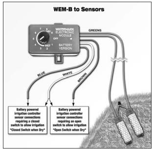
Run wires from the battery operated irrigation valve/controller's sensor connection to the WEM-B and make waterproof connections as follows (see wiring diagram).
