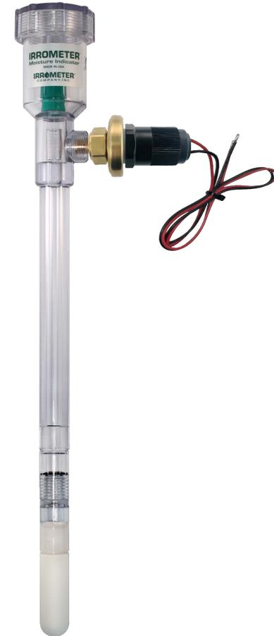
The Adjustable Vacuum Switch is mounted directly on the IRROMETER instrument body. It can be easily field adjusted to the desired soil moisture switching set point. Its function can be compared to that of a thermostat, allowing the controller (or solenoid valve) to operate when irrigation is desirable, or keeping it out of operation when there is no need to irrigate.
