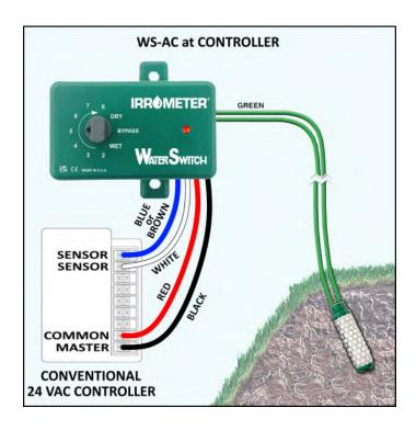
The WaterSwitch (AC) can be wired to a conventional 24 VAC controller, to a individual valve, or multiple switches can be wired to a single controller.
