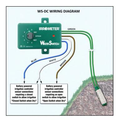
The WaterSwitch (DC) can be used with battery powered controllers equipped with a sensor circuit.
