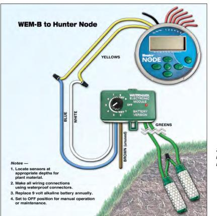
Shown here installed with Hunter valve/controller
