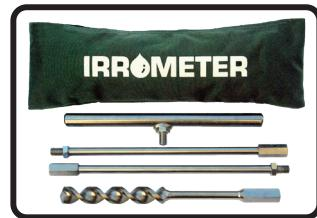
**Auger Tool Kit** – Nickel plated 1" (25 mm) soil auger. Makes oversize hole for grout style sensor installation in hard or rocky soils. Comes as a kit in fabric storage pouch with two 12" (30 cm) extensions and handle for making up to a 36" (90 cm) access hole. Cat #1014.....
