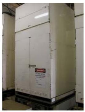
Phytotron used to carry out manipulation trial – allows control of temperature and light.
