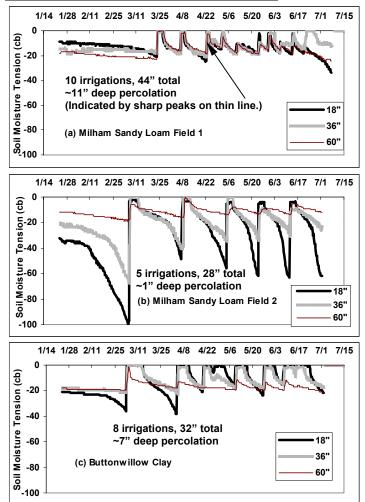
Fig. 7. Soil moisture "tension" changes during the 2002 season as measured by Watermark electrical resistance sensors and recorded every 8 hours with the AM400 data logger.
