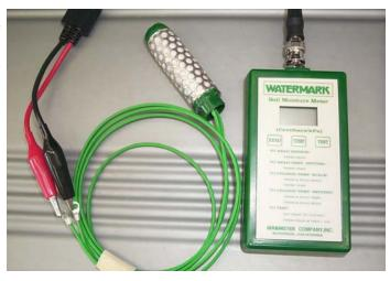
Electrical resistance block soil moisture probe with hand-held reader
