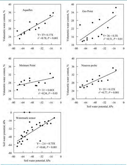
**Figure 3.** Soil water potential measured in Experiment 1 by tensiometers (X axis) regressed against soil moisture data (Y axis) measured by 5 types of soil moisture sensors. Data points for the Aquaflex sensor are the average of two sensors. Data points for the other sensors are the average of four sensors. Malheur Experiment Station, Oregon State University, Ontario, OR, 2001.
