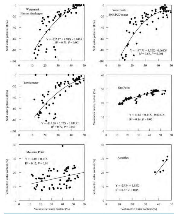
Figure 6. Volumetric soil water content measured in Experiment 2 by a neutron probe (X axis) regressed against soil moisture data (Y axis) measured by 6 types of soil moisture sensor. Malheur Experiment Station, Oregon State University, Ontario, OR, 2002.
