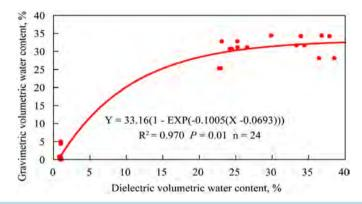
**Figure 10.** Regression of the volumetric soil water content measured by an ECH2O 10 dielectric aquameter (X axis) against the classical gravimetric method (Y axis). Data points from each of four ECH2O 10 dielectric aquameters were compared with two soil samples in each of three soil moisture ranges. Malheur Experiment Station, Oregon State University, Ontario, OR, 2004.
