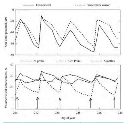
**Figure 1.** Soil moisture data over time for five types of soil moisture sensors in Experiment 1. Arrows denote irrigations with 50.8 mm of water applied. The Moisture Point sensor was not available during this time due to repairs being made. Malheur Experiment Station, Oregon State University, Ontario, OR, 2001.
