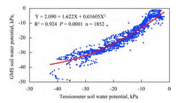
**Figure 8.** Soil water potential measured in Experiment 3 by a tensiometer with transducers (X axis) regressed against soil moisture suction measured by a granular matrix sensor (Y axis). Data points are the average of eight instruments. Malheur Experiment Station, Oregon State University, Ontario, OR, 2004.
