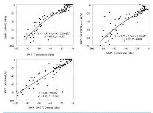
**Figure 5.** Regressions of soil water potential (SWP) measured in Experiment 2 by three instruments. Malheur Experiment Station, Oregon State University, Ontario, OR, 2002.
