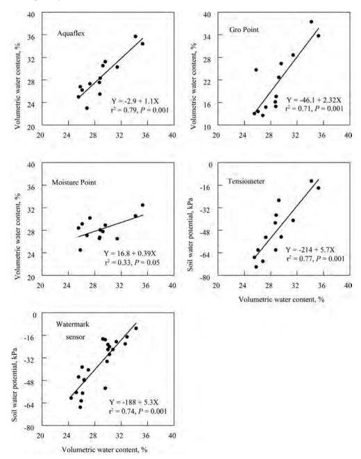
**Figure 2.** Volumetric soil water content measured in Experiment 1 by a neutron probe (X axis) regressed against soil moisture data (Y axis) measured by 5 types of soil moisture sensors. Data points for the Aquaflex sensor are the average of two sensors. Data points for the other sensors are the average of four sensors. Malheur Experiment Station, Oregon State University, Ontario, OR, 2001.
