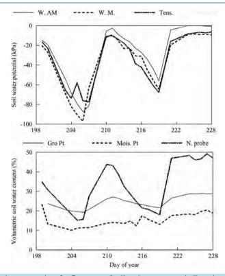
**Figure 4.** Soil moisture over time for five types of soil moisture sensors in Experiment 2, tensiometers (Tens.), Watermark soil moisture sensors read by a AM400 datalogger or manually (W. AM or W. M.), Gro Point (Gro Pt), Moisture Point (Mois. Pt) and neutron probe (N. probe). Malheur Experiment Station, Oregon State University, Ontario, OR, 2002.
