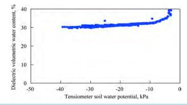
**Figure 9.** Soil water potential measured in Experiment 3 by a tensiometer with transducers (X axis) regressed against volumetric soil water content measured by an ECH2O 10 dielectric aquameter (Y axis). Data points for soil water potential are the average of eight tensiometers. Data points for the ECH2O 10 dielectric aquameter are the average of four sensors. Malheur Experiment Station, Oregon State University, Ontario, OR, 2004.
