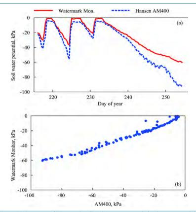
Figure 11. Response of Watermark soil moisture sensors to irrigation events and the termination of irrigation as measured by a Hansen AM400 datalogger and an Irrometer Watermark Monitor in Experiment 4. The average readings of an AM400 datalogger and a Watermark Monitor are compared over time (a) and over the measured range of soil water potential (b). Malheur Experiment Station, Ontario, OR, 2003.
