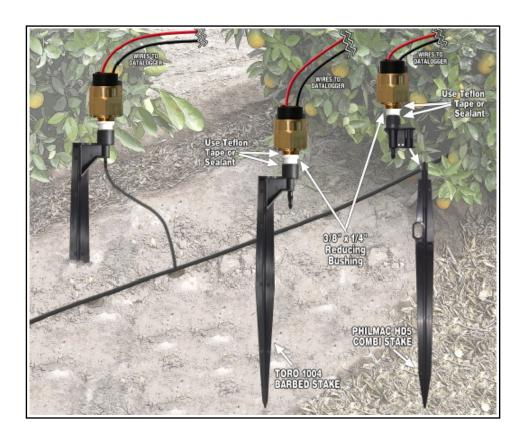
The diagram here shows an example of a typical field installation using commercially available stake and pipe fitting assemblies (not available from IRROMETER), making an easy way to attach the PPS to a drip irrigation tubing system.
