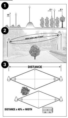
reduce the radio range. The operating range will also be reduced if the Nodes are not installed at adequate heights. (see Figures 2 & 3)
