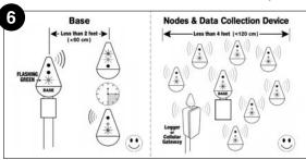
If associating a large number of Nodes, do so in batches of 8-10 at a time. Once each batch is done. turn off the Base, move the first batch of Nodes far enough away (3000'+ [915 m]) so the Base can't 'hear' them anymore, then restart the Base and associate the next batch, A data collection device (Logger, PC Link or Cellular Gateway) is counted as a Node for purposes of association.
