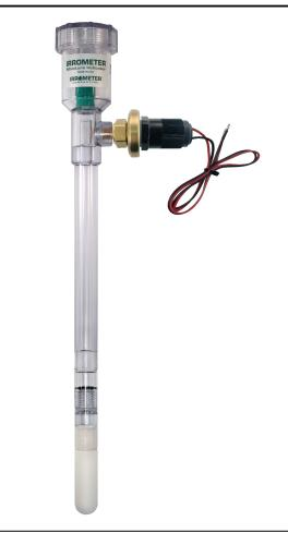
The Adjustable Vacuum Switch is mounted directly on the IRROMETER instrument body. It can be easily field adjusted to the desired soil moisture switching set point. Its function can be compared to that of a thermostat, allowing the controller (or solenoid valve) to operate when irrigation is desirable, or keeping it out of operation when there is no need to irrigate.
