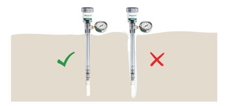
Push the IRROMETER into the prepared hole. Always handle by the cap or reservoir- do not push or pull on the gauge. Avoid twisting the instrument counterclockwise while installing as this can loosen the replaceable tip. Once installed, mounding a few inches of soil around the instrument will create drainage to prevent pooling.
