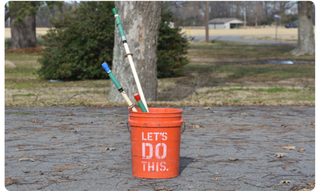
Figure 3. Soak sensors preferably in the irrigation water that will be applied to the field or fresh rainwater; however, tap water also can be used.
