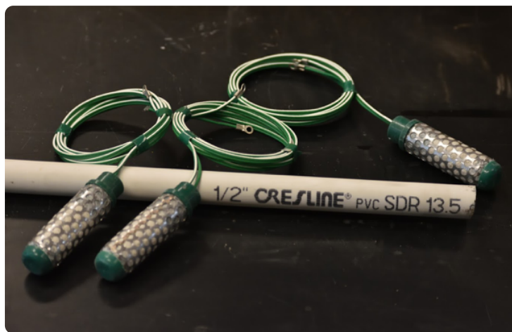
Figure 1. The sensor is attached to a length of PVC pipe which facilitates installation to the desired depth in soil. The 1/2-inch SCH 20 PVC pipe (315 PSI, thin wall ASTM D2241) is the right size to provide a snug fit with the Watermark sensor collar. Do not use ordinary 1/2-inch PVC pipe.
