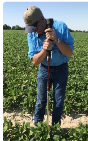
Figure 3. Sensors should be installed early in the season when plants are small so that the installation does not damage roots. Plants with roots that are damaged by sensor installations may not use water the same as undamaged plants.
