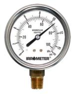
Glycerin filled for severe service conditions with pulsation and vibrations. Features stainless steel case with durable 2 1/2 in. (63mm) polycarbonate face. Connected with a 1/4 in. brass standard pipe thread stem (NPT) and integral snubber. Dual scale P.S.I. and kPa faceplate.
